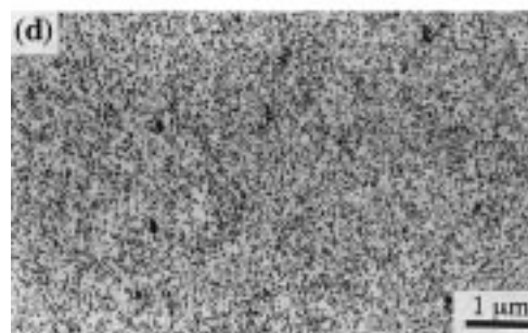
Fig. 4. TEM micrographs of 20/80 PSU/PA blends melt-mixed at 260°C for 8 min (rotor speed; 100 rpm): (a) nf-PSU/PA, (b) PSU-triazine/PA, (c) PSU-epoxy/PA, and (d) PSU-PhAH/PA.
